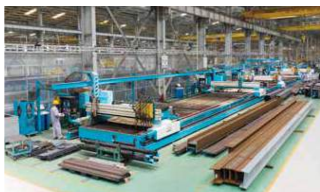
CNC GAS & PLASMA CUTTING MACHINE Thickness: 150 mm Cutting size: 3,200 x 15,000 mm
