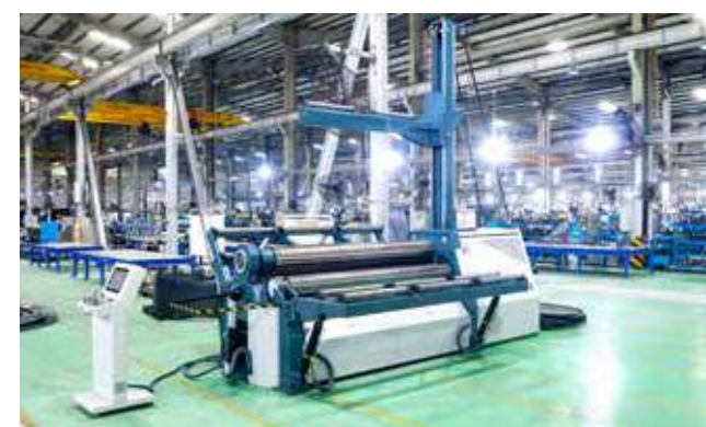
CNC PLATE ROLLING MACHINE Maximum length: 2,550 mm Diameter axes: 300 mm Maximum thickness: 13 mm
