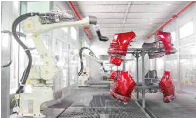
ROBOT PAINTING Quantity: 5 robots Capacity: 160,000 sets/year
