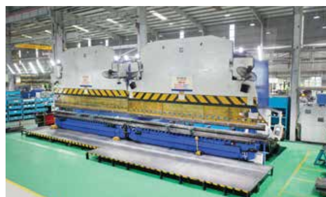
CNC PRESSING MACHINE (12M) Thickness: 0.6 - 12 mm Workable length: 12,000 mm
