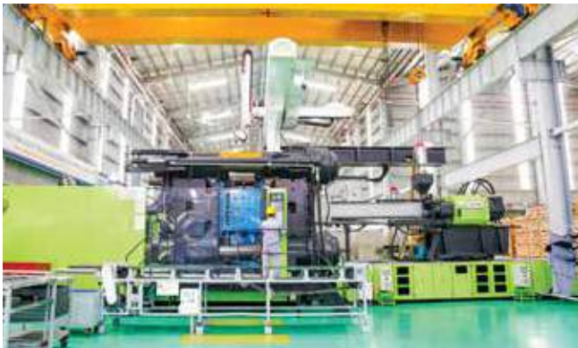
3,200 TONS INJECTION MACHINE Injection pressure: 200 Kg/cm² Productivity: 120,000 products/year
