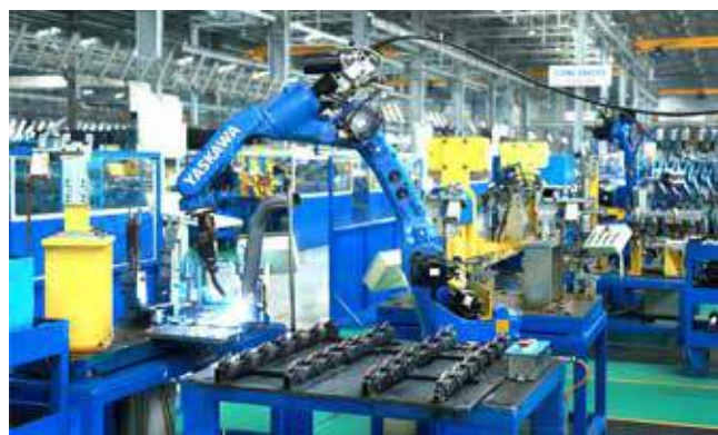
WELDING ROBOT LINE Quantity: 63 machines Gas metal arc welding Flux cored arc welding
