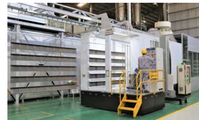
POWDER COATING LINE Load: 140 kg Max material size: 5,500m x 2,000 x 600 mm
