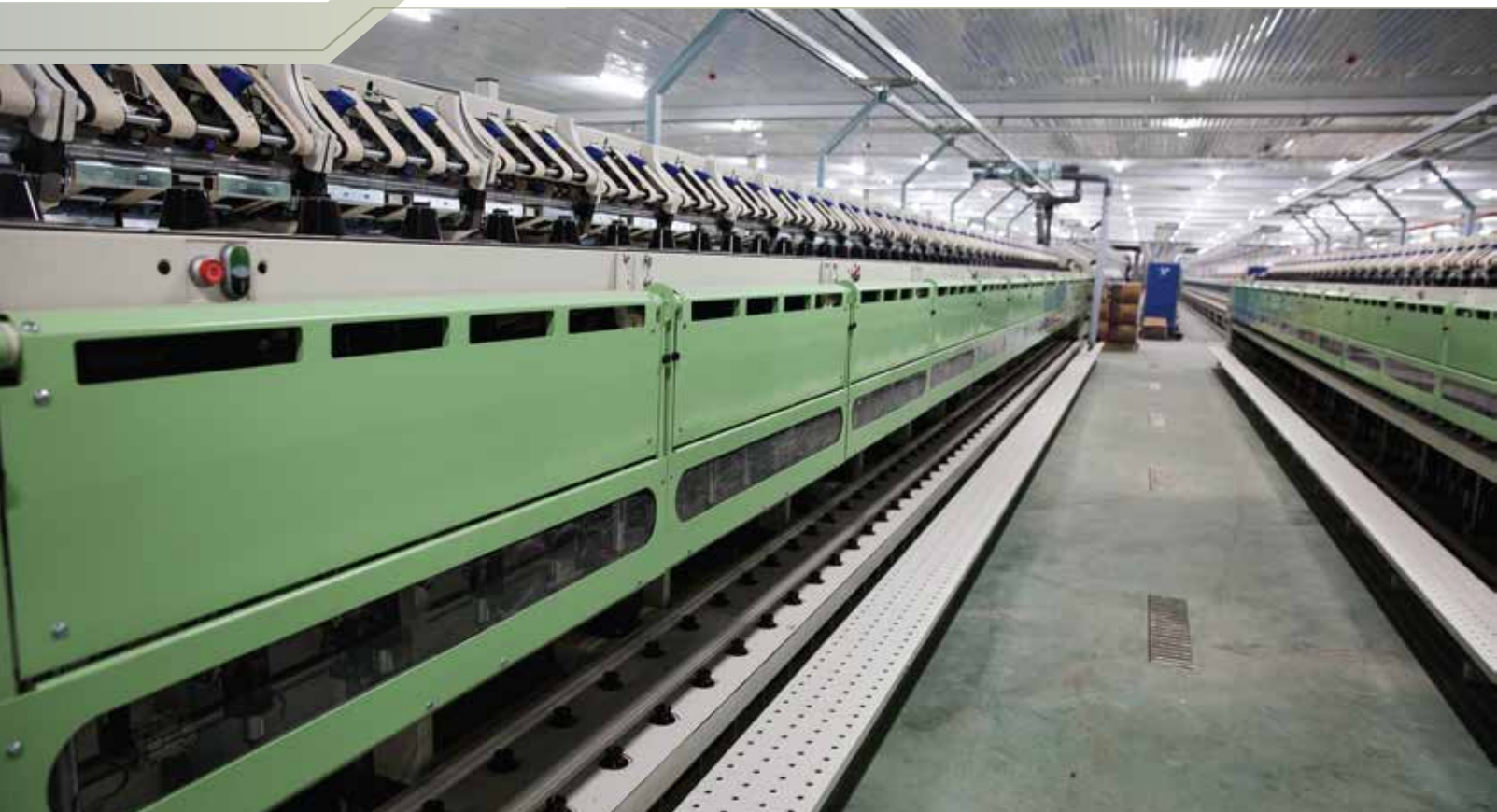
Máy kéo sợi thô Lakshmi Model LF4200A Speed frame LF4200A
