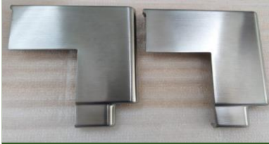
6.5 Hard Chrome coating on Steel
