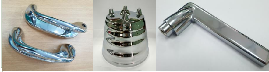
6.3 Cu-Ni-Cr coatings on Zinc with Hairline
