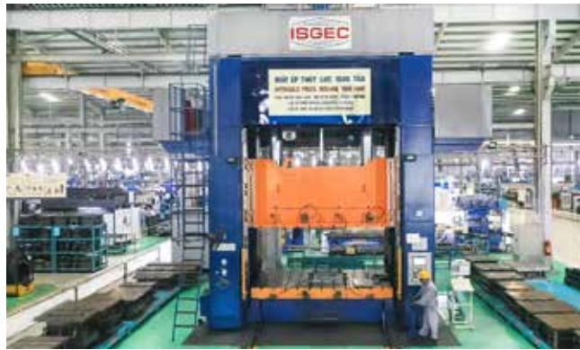
HYDRAULIC PRESS MACHINE 1,000 TONS Press force: 1,000 tons Working table size: 3,500 x 2,200 mm
