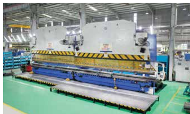
CNC PRESSING MACHINE 12 METERS Thickness: 0.6 - 12 mm Workable length: 12,000 mm
