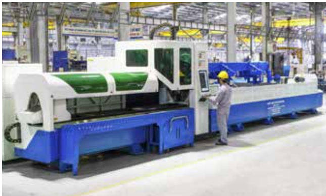
SQUARE STEEL, TUBE STEEL LASER CUTTING MACHINE Thickness: 8 mm (steel); 4 mm (inox) Cutting size: Ø20 – 220 mm; □15 - 155 mm
