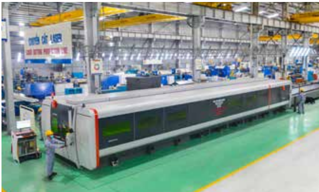
FIBER LASER CUTTING MACHINE Quantity: 04 machines Thickness: 25 mm Cutting size: 12,300 x 2,000 mm
