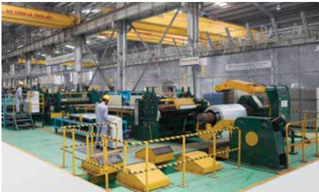
SLITTING LINE Quantity: 03 lines Thickness: 0.3 - 6 mm Width: 50 - 1,200 mm
