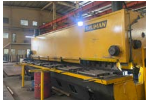
Steel plate cutting machine 16mm-4m
