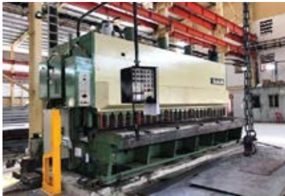
Steel plate cutting machine 22mm - 6m
