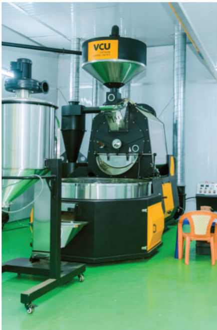
The 12kgs and 60kgs hot air coffee roaster machine
