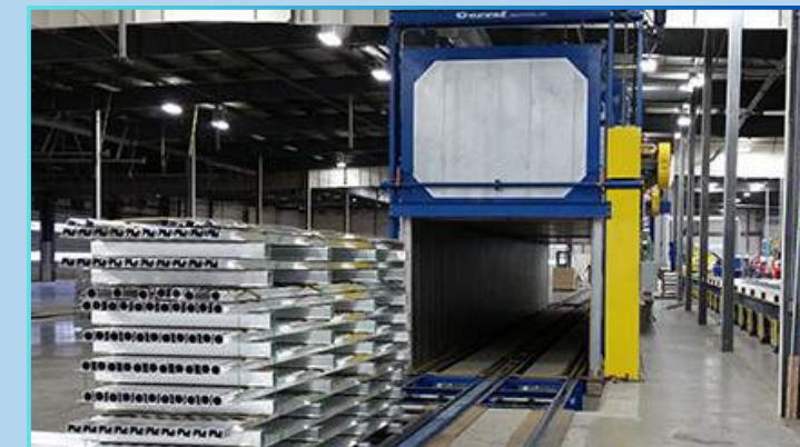
PLC cycle aging oven
