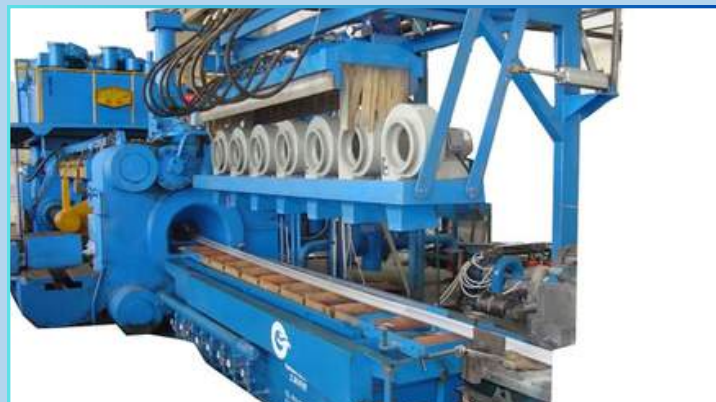
Water and air control in-line-quenching system
